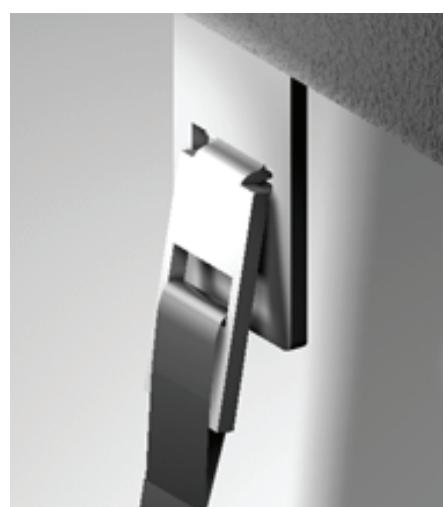
STEP 1: Locate the sidewall or longitudinal bracket installed by home manufacturer, insert Quick Connector into bracket slot at 45 degree angle.
