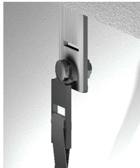
STEP 1: Locate the sidewall or longitudinal bracket installed by home manufacturer, insert bolt through hole in Quick Connector then through hole in bracket.
