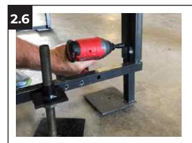
Once in position, secure the **H Brace (C)** to the **Adjustable Leg (A)** with one 14 x 14 x 3/4 Tek screw in the pre-drilled pilot hole near the bottom of the **H Brace (C)**.
