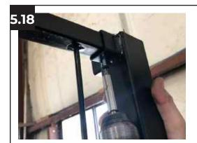
Secure all deck rails with a single #10-16 x 1" Phillips head screw through the underside of the top post sleeves, and the top of the bottom post sleeves.
