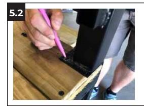
Line up the hole in the front of the post bracket with the pre-drilled hole in the frame of the **Platform Module (D)**. Once positioned correctly, mark the location of the hole in the top of the post bracket.
