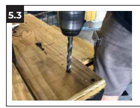
Use the mark as a guide to drill a pilot hole through the **Platform Module (D)**. Once drilled, reposition the post in place.
