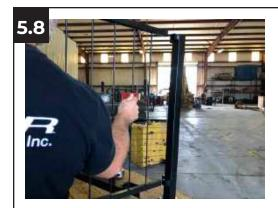
Insert the **58 3/4" Deck Rail (K)** section into the sleeves located on the side of the first **Corner Post (J)**.
