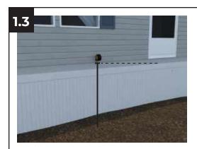
Beginning from the point established in the previous step, measure down from where the edge of the steps will be located to the ground.
