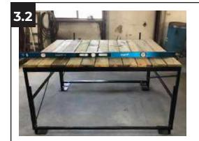
Using a carpenters level, verify that the top of the deck is level in both directions.
