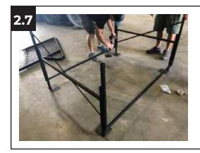
Repeat the previous two steps on the remaining Adjustable Legs (A), using a carpenters level to ensure the top of each H Brace (C) is level before securing to the Adjustable Legs (A).
