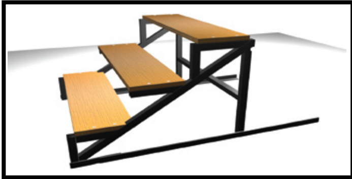
3. Insert the 24" H Brace (P#1) into sleeves and rest on 1x1 angle iron base rail.
